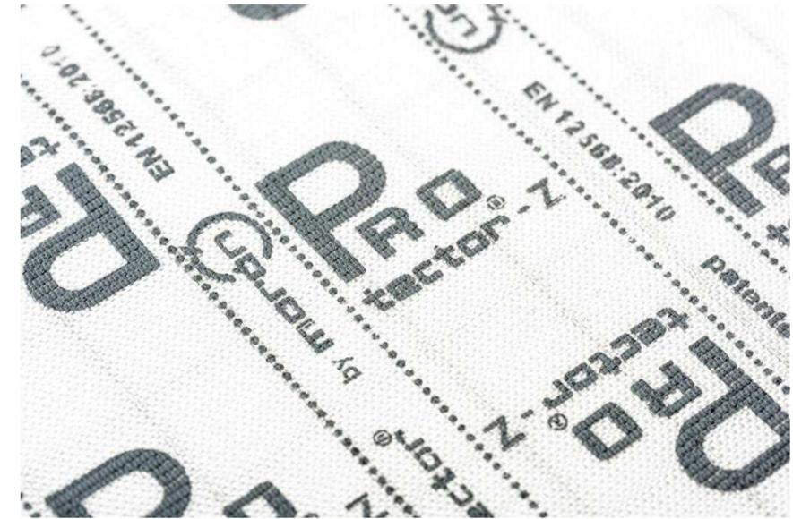
In our safety footwear, puncture resistance is secured with KEVLAR lining midsole instead of steel plates. The midsole which complies with the EN ISO 20345 Standard, prevents any kind of penetration of a nail width of 4.5 mm and a force of 1100 Newton.
